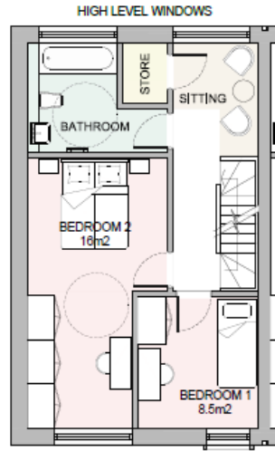
27 First Floor Plan 1:50
